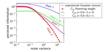
If a = 0, b = 0 and c = 1 the degree of the leakage function is 3, hence the slope of the IT curve is  $\frac{4}{3}$ .
