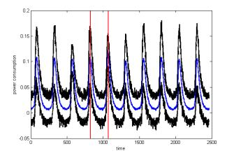
Protected software device with 2 shares: ideally bidimensional leakages are sufficient to mount an attack.
