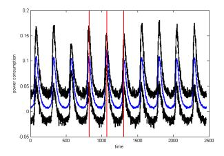
Protected software device with 3 shares: ideally tridimensional leakages are sufficient to mount an attack.
