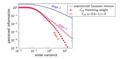
If a = 0, b = 1 and c = 0 the degree of the leakage function is 2, hence the slope of the IT curve is  $\frac{4}{2}$ .
