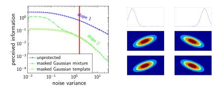
For unprotected device difference is still in the mean. For protected full distribution and Gaussian template model are close  $\Rightarrow$  few information in higher order.
