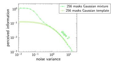
Using Gaussian mixture allows us to obtain more information for low noise.  $\exists$  useful information in higher moments that gradually vanishes as noise increasing.
