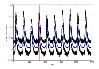
Unprotected device: unidimensional leakage is sufficient to mount an attack.
